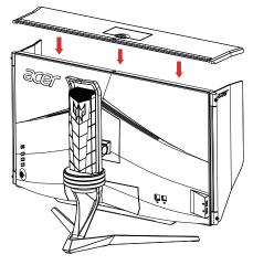
5. Shading hood installation complete.
