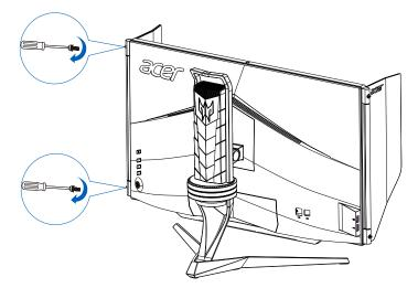
4. Put down top shield and fix on the head.
