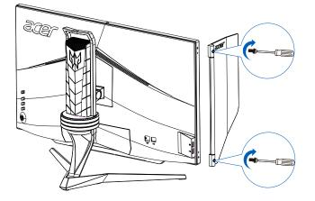
2. Use screwdriver or coin to fasten screw and fix door on the head.
